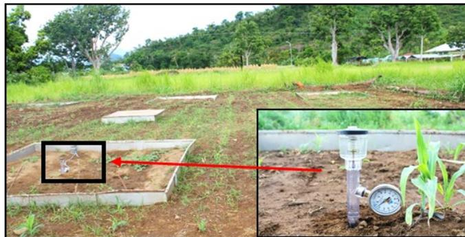
Figure 3. Tensiometer installed inside lysimeter tank.
