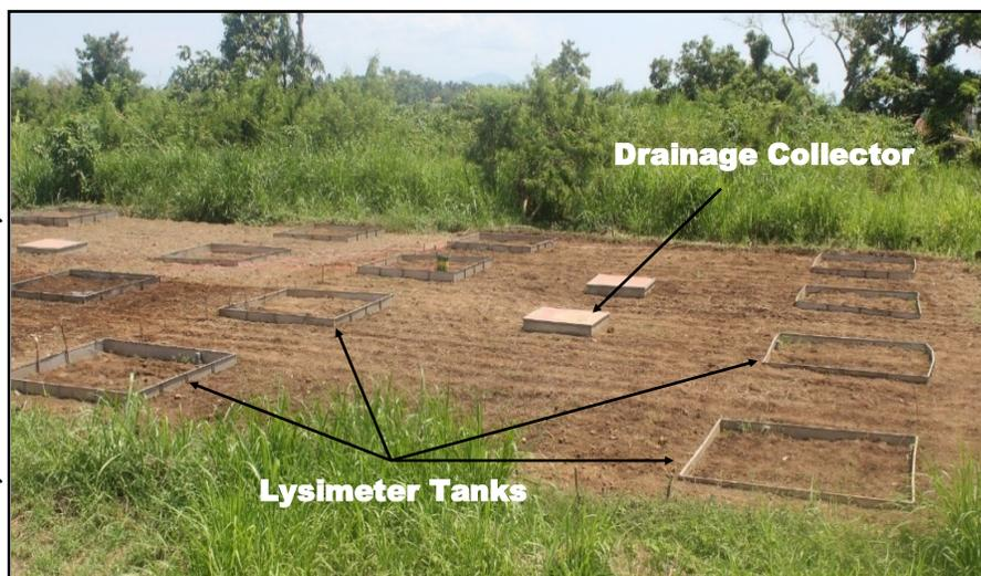
Figure 2. Lysimeter Setup.
