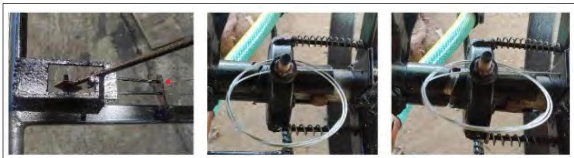
Figure 3. Clutch lever (left) engaged clutch (middle), and disengaged clutch (right) of the seeder.
